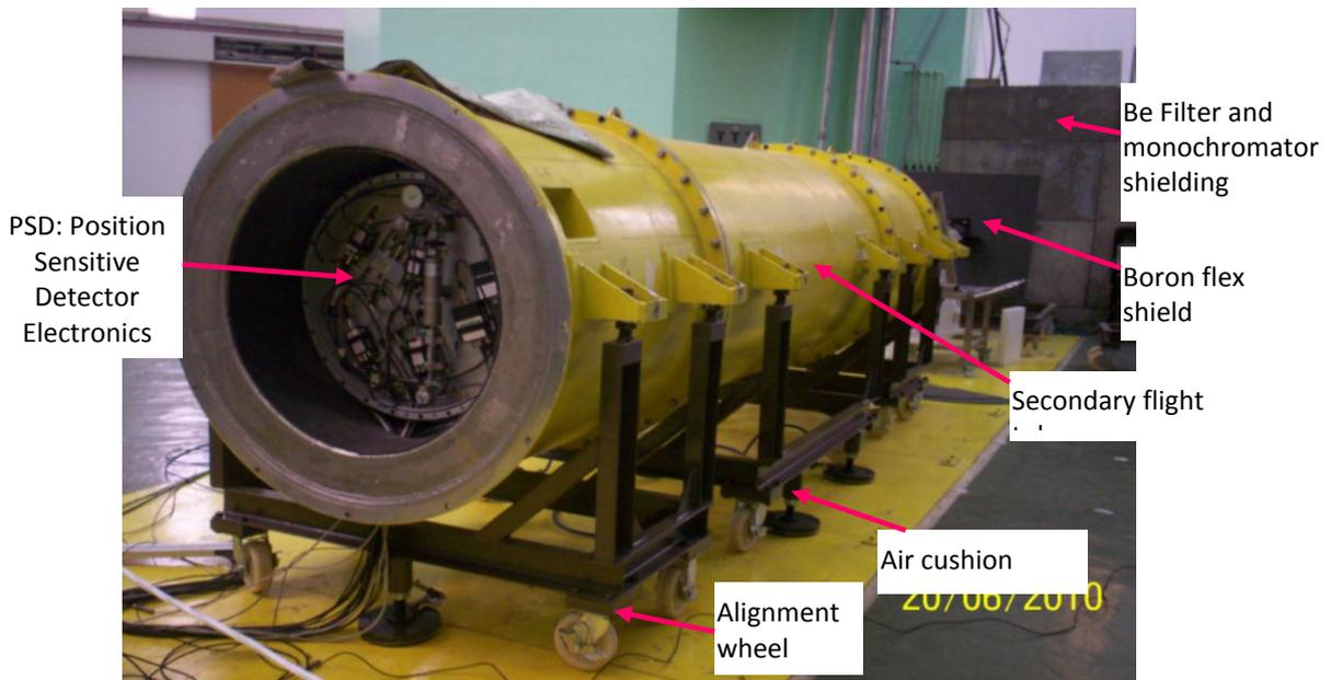
Fig. 4. SANS facility at the Reactor TRIGA PUSPATI in Nuclear Malaysia.
