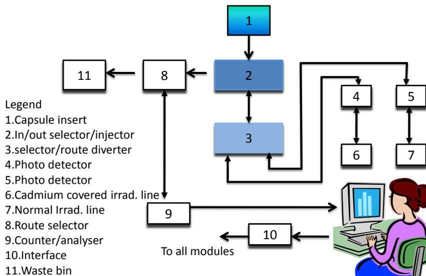
Fig. 2. Block diagram of the Delayed Neutron Analysis (DNAA).
