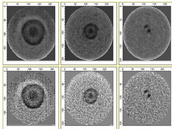
Fig. 8. Results of reconstruction of the spark plug.
