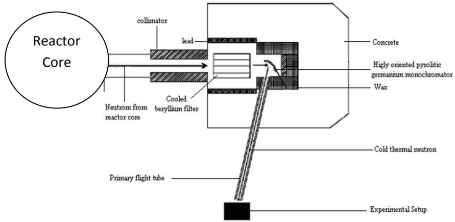
Fig. 3. Schematic design of SANS set-up.
