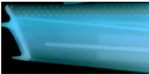
Fig. 11. Neutron radiographic image of a used turbine blade.
