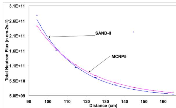
Fig. 14. Comparison of neutron fluxes between SAND-II and MCNP at the centre of thermal column.
