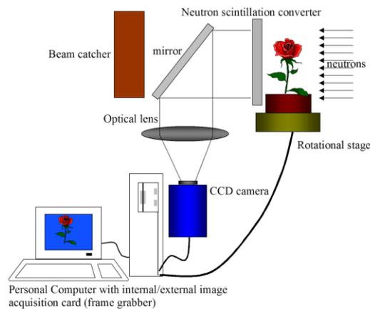
Fig. 10. Schematic set-up of the digital neutron radiography.
