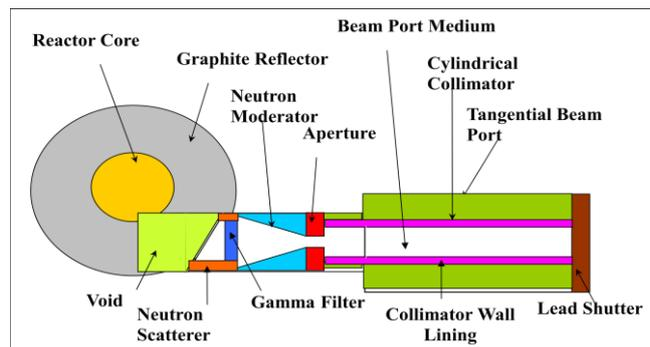
Fig. 12. Final design of The optimized neutron collimator for tangential beamport of RTP.
